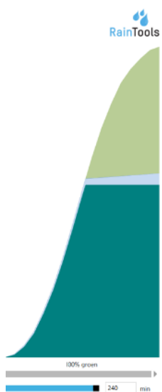
A15 Water balance of hypothetical gardens (consisting of 0-100% grass) in time (180 min) the custom precipitation event (drizzle), showing the increase in infiltration & storage in the soil and the decrease in the runoff & storage on the surface when the greening of the gardens enhances.
