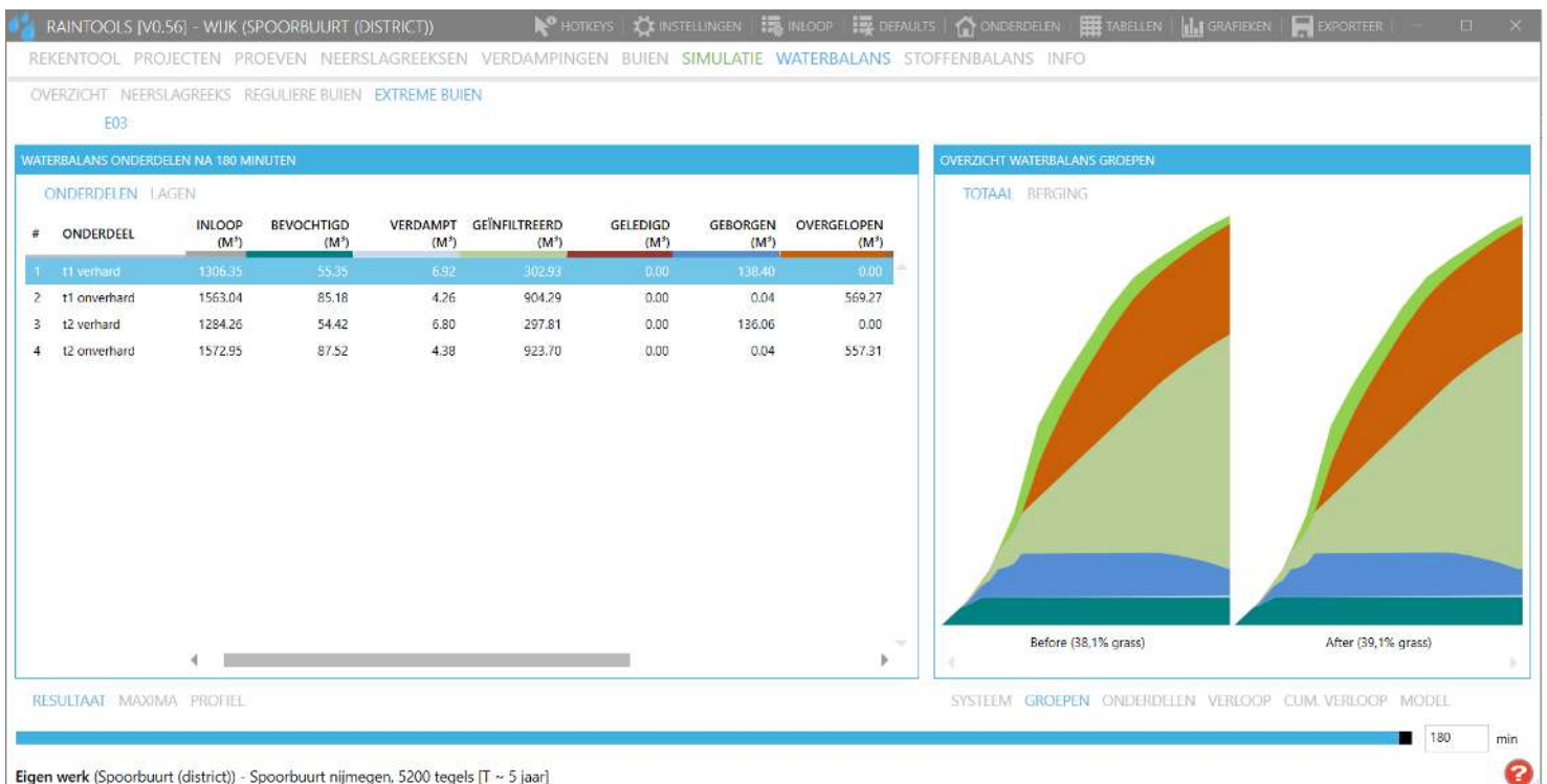
Figure 10 Output window of the Wijktegel for a simulation of the Spoorbuurt district before and after the greening during E03. The graphs depict the different terms of the water balance table in respect to time (180min). The colours correspond to the terms in the table which also lists their volumes in m 3 for each layer that is defined in the model.
